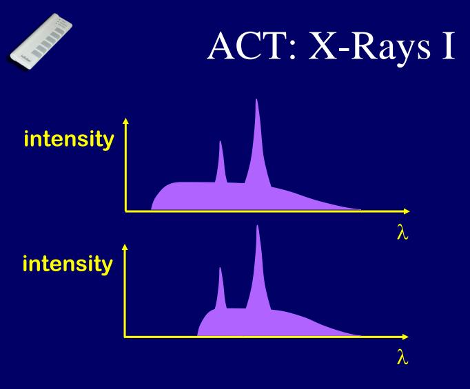
Which graph corresponds to the tube being operated at the higher voltage?
