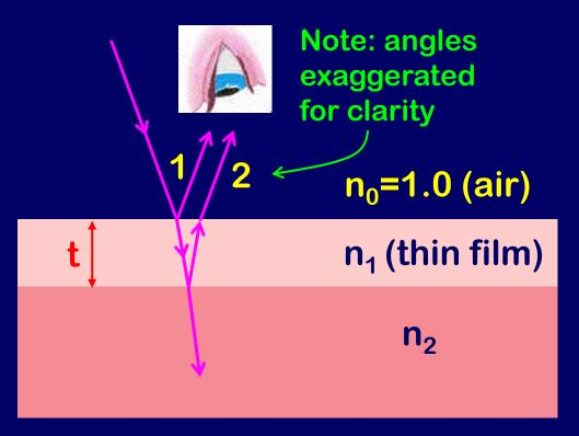
Get two waves by reflection off two different interfaces: interference! Ray 2 travels approximately 2t further than ray 1.
