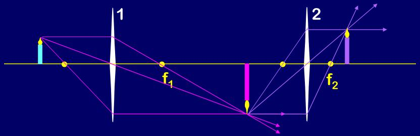
Lens 1 creates a real, inverted and enlarged image of the object.
