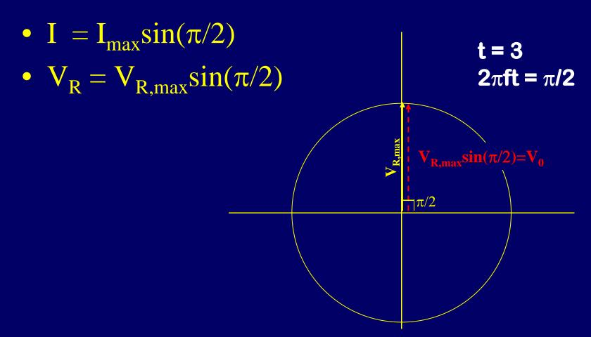
Length of vector = V<sub>max</sub> across that component Vertical component = instantaneous value of V
