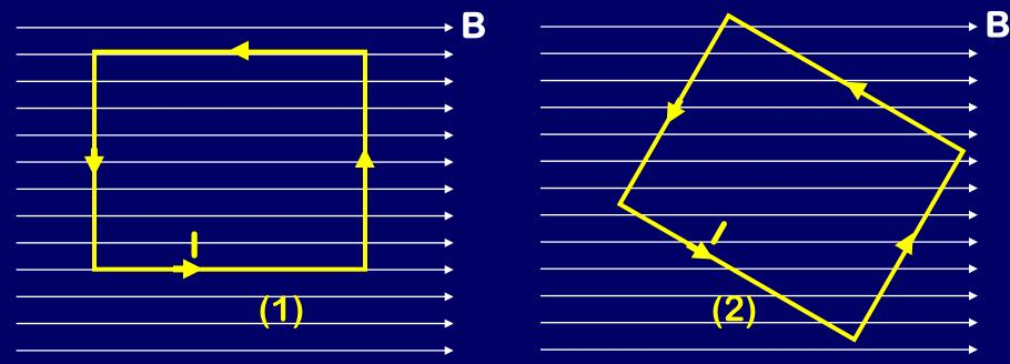
Compare the torque on loop 1 and 2 which have identical area, and current.
