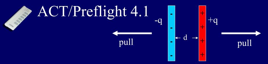
A parallel plate capacitor given a charge q. The plates are then pulled a small distance further apart. Which of the following apply to the situation after the plates have been moved?
