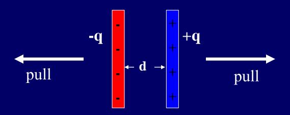
A parallel plate capacitor given a charge q. The plates are then pulled a small distance further apart. What happens to the charge q on each plate of the capacitor?
