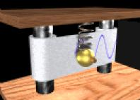
A 3 kg mass is attached to a spring (k=24 N/m). It is stretched 5 cm. At time t=0 it is released and oscillates.
