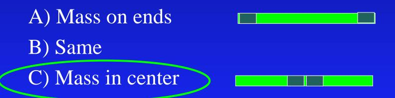
$I = \Sigma m r^2$  Further mass is from axis of rotation, greater moment of inertia (harder to spin)
