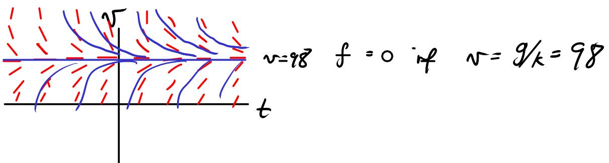
All solution curves asymptote to the constant solution  $v = 98 \text{ m/s}$  ← called terminal velocity.
