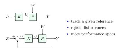
Intuitively, the difference between the open-loop and the closed-loop architectures is clear (think cruise control ...)
