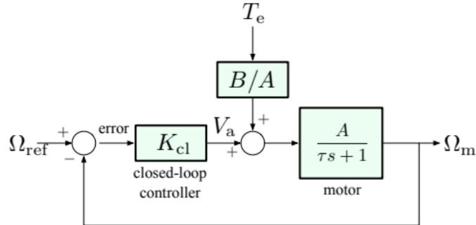
$$\Omega_m = \underbrace{\frac{AK_{\text{cl}}}{\tau s + 1 + AK_{\text{cl}}}}_{\text{DC gain} = \frac{AK_{\text{cl}}}{1+AK_{\text{cl}}}} \Omega_{\text{ref}} + \underbrace{\frac{B}{\tau s + 1 + AK_{\text{cl}}}}_{\text{DC gain} = \frac{B}{1+AK_{\text{cl}}}} T_e$$
