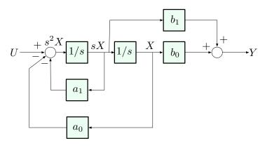
Can we write down a state-space model corresponding to this diagram?
