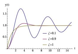
The parameter  $\zeta$  is called the damping ratio
