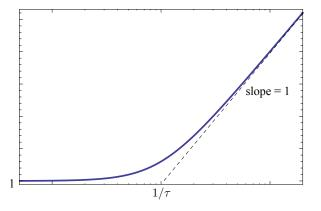
For a stable real zero, the magnitude slope "steps up by 1" at the break-point.
