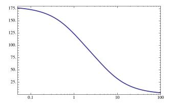
For a RHP zero, the phase plot is similar to what we had for a LHP pole: goes down by  $90^{\circ}$  ... However, it starts at  $180^{\circ}$ , and not at  $0^{\circ}$ .
