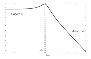
For a stable real pole, the magnitude slope "steps down by 2" at the break-point.
