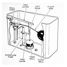
The flush toilet employs a control mechanism that ensures that the toilet gets flushed and that the tank is filled to a set reference level. Similar systems are used in other applications where fluid levels need to be regulated.
