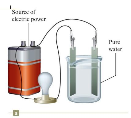
Pure water does not conduct an electric current. The lamp does not light.
